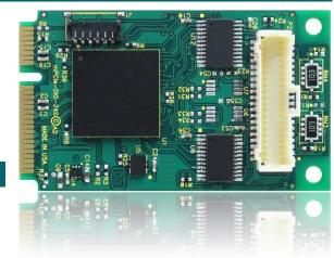
The mPCle-II-16 consists of a type F1 PCl Express Mini Card (mPCle) interface board that connects to a Mobile-ITX-sized, DB-37M Isolation Module via an included 9" cable. That module is designed to be easily panel-mounted in any application environment. It uses the high speed PCl Express bus to transfer digital data to and
